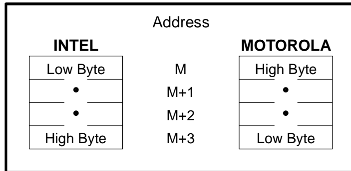
Figure 4-1 Byte Ordering Schemes
